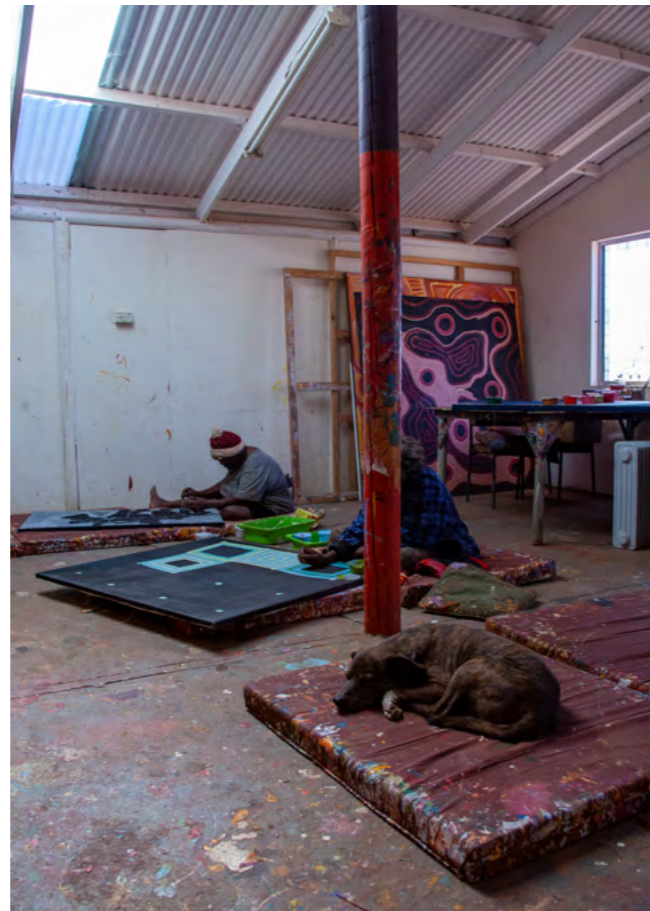
↑ The studio extension provides a protected and private space for artists to work with good daylight provided by polycarbonate 'skylights'. However, with no external shading, the single layer skylights make the room subject to high temperatures.
